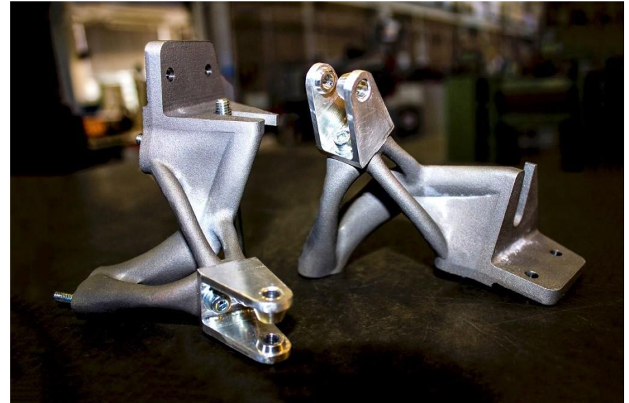
Figure 5: AM is an evidence in projects where optimization is pushed to its limits, like these titanium brackets manufactured with SLM, from Formula Student Team TU Delft [2]
