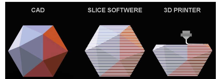
Figure 11: Slicing of a CAD model into layers
